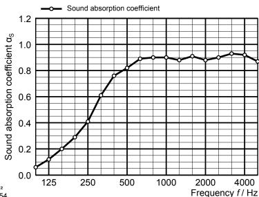
$<sup>\</sup>circ$  Equivalent sound absorption area less than 1.0  $\text{m}^2$   $\alpha_{\text{S}}$  Sound absorption coefficient according to ISO 354
