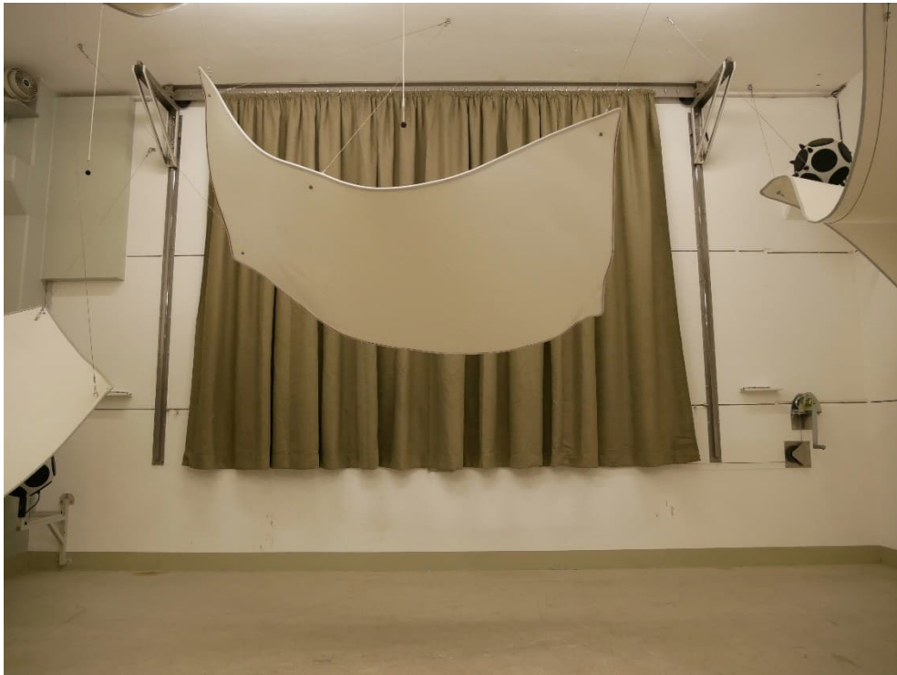
Figure B.1. Pleated hanging curtain in the reverberation room (frontal view).
