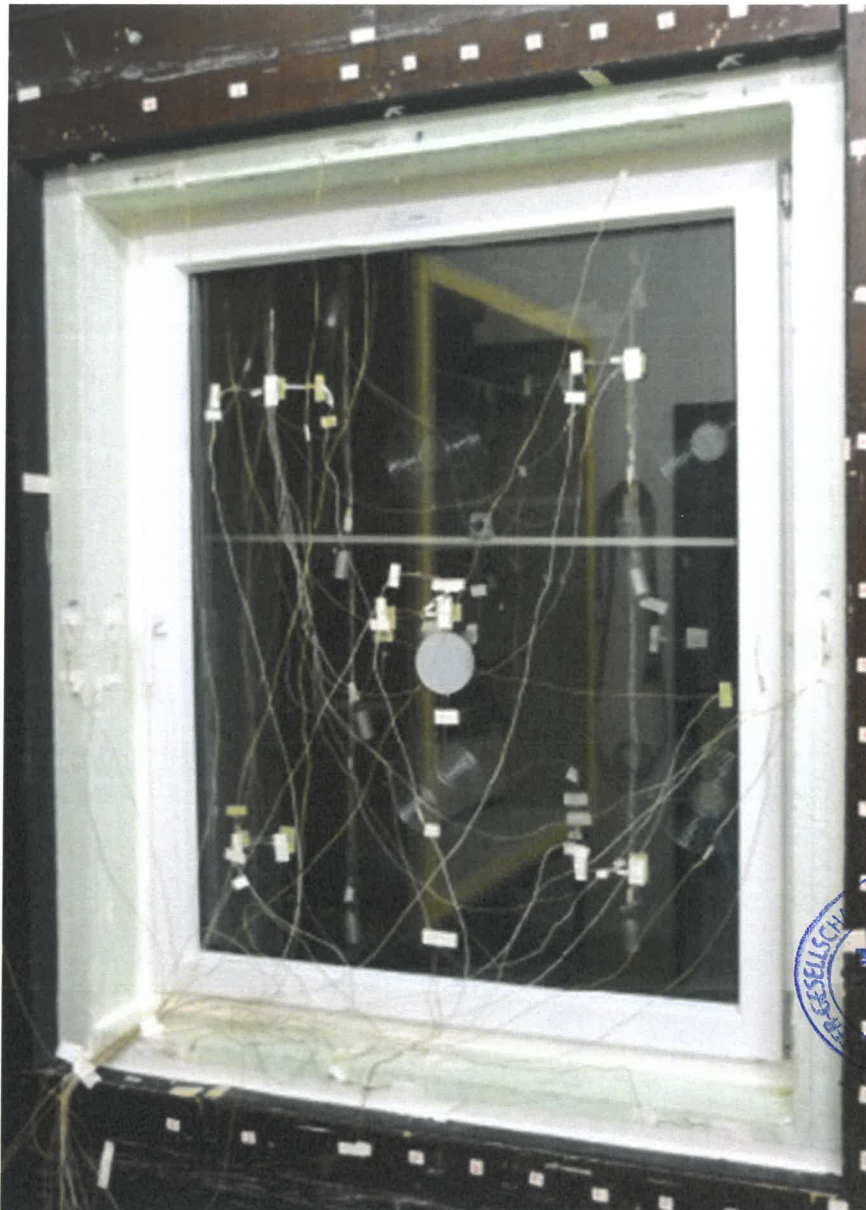
Figure 2: Test setup of section 2, inside view: window without curtain [1] and [2].
