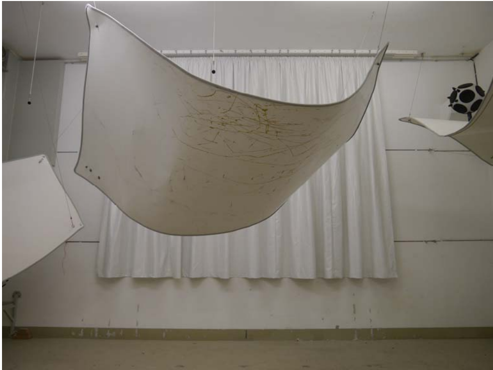
Figure B.1. Test object in the reverberation room: frontal view.
